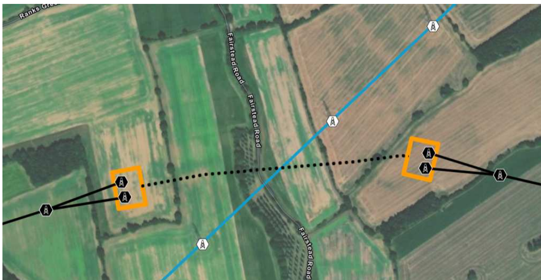
Figure 1: Black solid = new proposed overhead lines, black dash = new proposed underground cables, black hexagon = proposed new pylon, blue solid = existing overhead line, white hexagon = existing pylon. Source: National Grid Interactive Map.
