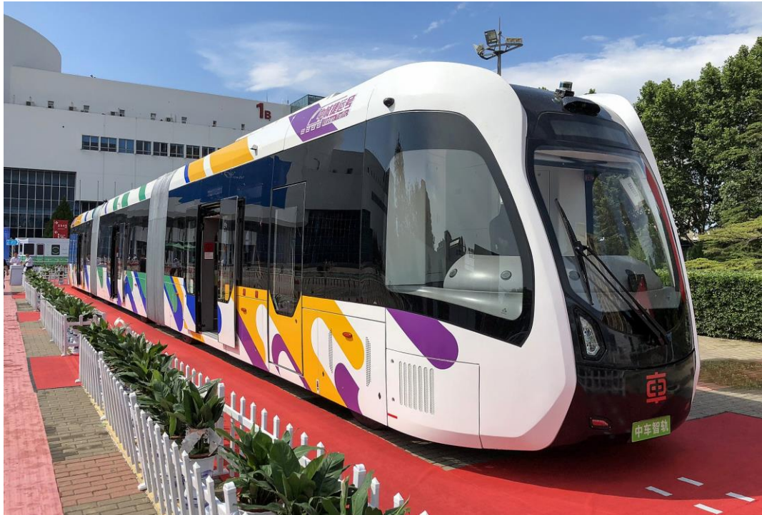
Figure 2-3: “Trackless trains” – self-driving vehicles, which have the rubber-wheels of a bus, use sensor technology to follow markings painted on the streets.
